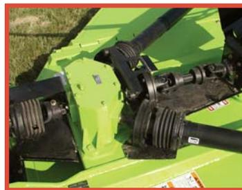
**Forward Mounted Slip Clutches**
